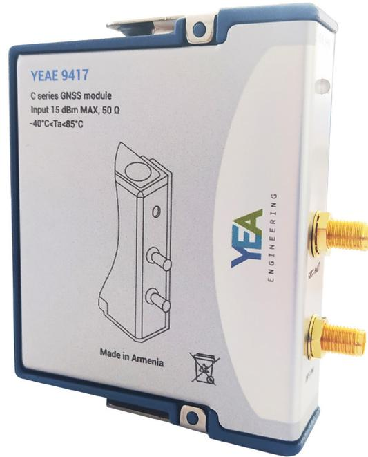
The YEAE 9417 is a concurrent GNSS receiver module for NI C series platforms. It can receive multiple GNSS systems signal (e.g GPS/QZSS, GLONASS, BeiDou). Due to dual-frequency RF front-end architecture, two of the three signals (GPS L1C/A, GLONASS L1OF, and BeiDou B1) can be received and processed simultaneously.
